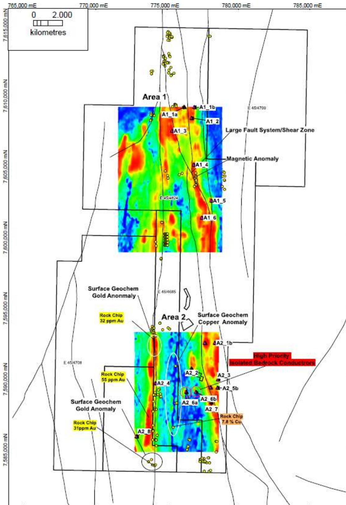
Figure 1. Hillside SkyTEM survey flown at 150 m line spacing showing conductors and geochemical anomalies.
